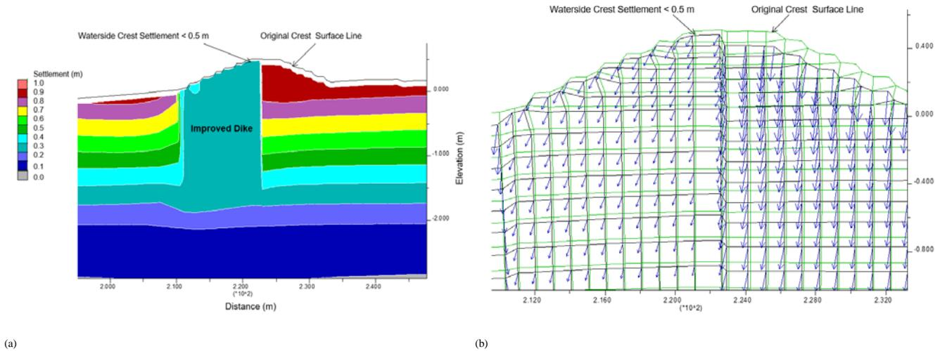
Figure 3. Computed Post-Earthquake Dike Settlement Pattern with Ground Improvement: (a) Displacement Contours after Settlement, (b) Distorted Mesh around the Crest after Settlement.
