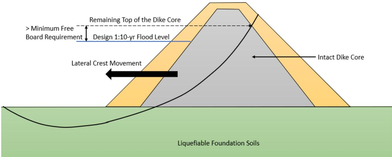
Figure 4. A Schematic Diagram Illustrates the Water Retaining Capacity of the Landside Dike Core is Functional after Waterside Dike Core is Comprised
