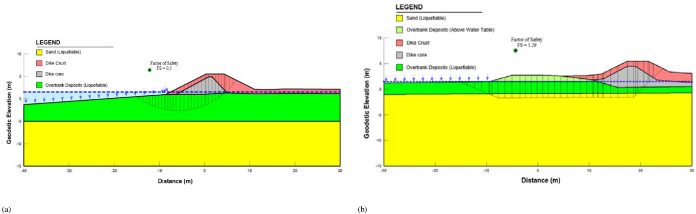
Figure 2. Post-Liquefaction Stability of Dike Segments: (a) Segment-1 (Sloping Ground Towards Waterside –  $FOS_{flowslide} < 1.0$ ), (b) Segment-2 (Buttressed Towards Waterside –  $FOS_{flowslide} > 1.0$ ).
