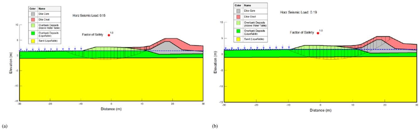
Figure 5. Computed Yield Acceleration for Dikes: (a) for the Movement of Waterside Slope (Dike Core Undisturbed), (b) For the Movement of Landside Slope (Dike Core Disturbed, However the Flood Protection not Compromised).
