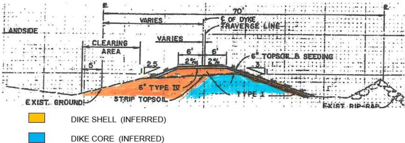
Figure 1. Typical Dike Cross Section
